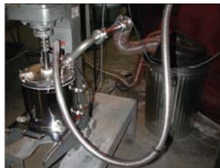
Figure 5. Vapor recovery system and special mill covers must be used with cryogenic milling.
