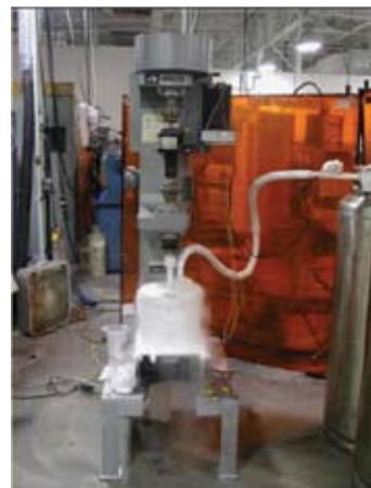
Figure 4. A research attritor being used with a cryogen.
