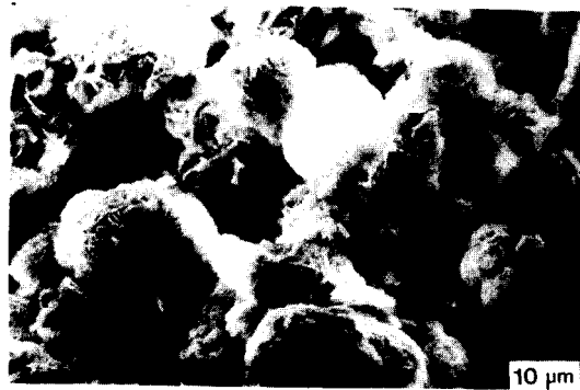
Figure 1. SEM photomicrographs of the component powders 'a'-PbCO 3 , 'b'-Nb 2 O 5 , and 'c'-MgCO 3 .
