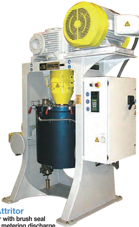
SD-30 Attritor Sealed cover with ceramic-lined tank, zirconium oxide sleeved arms, and actuated discharge assembly. Explosion-proof electricals.
