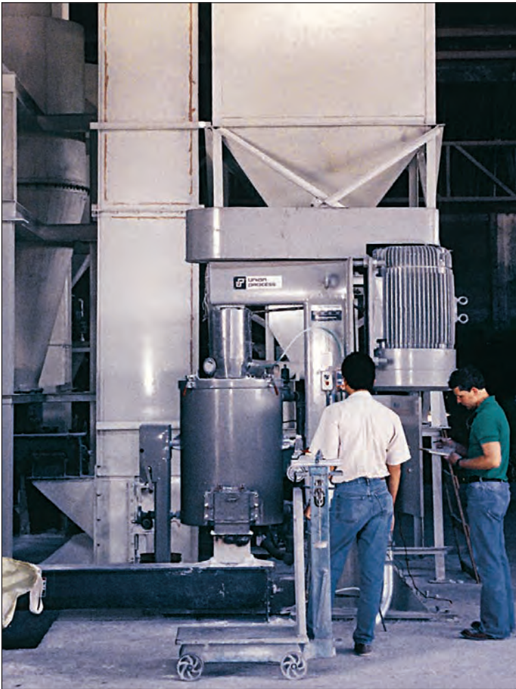
Installation of an HSA-100 for continuous fine dry grinding of calcium carbonate and barites.
