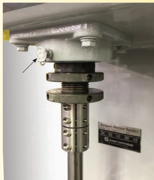
Adjustable Agitator Shaft Detail
