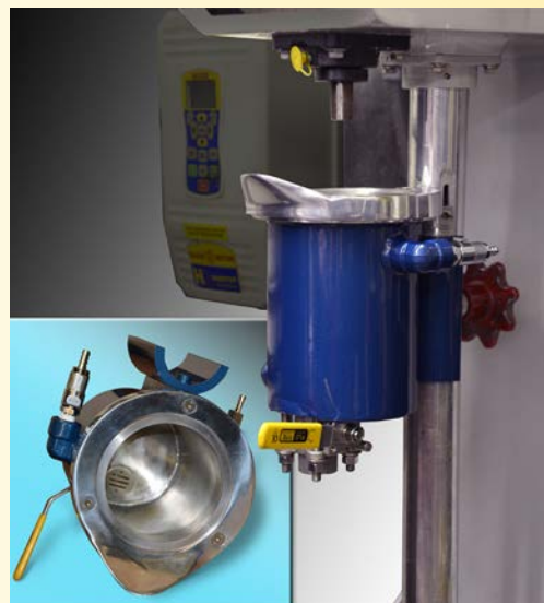
One-piece tank showing bottom discharge grid and valve.
