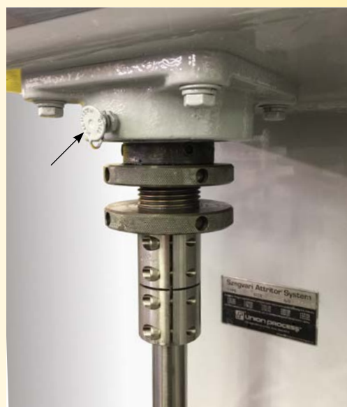
Adjustable Agitator Shaft Detail
