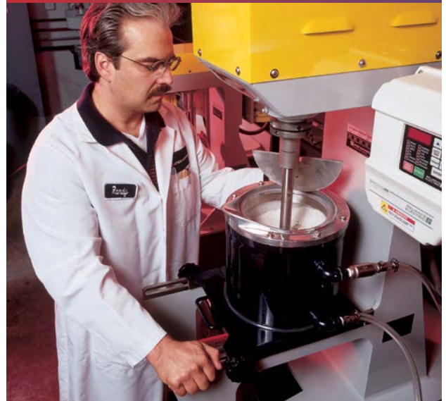
S-1 Attritor with variable frequency drive and 3 HP motor.
