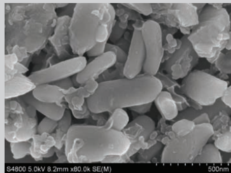
SEM (0.5µ) of lithium iron phosphate after processing for 0.5 hr
