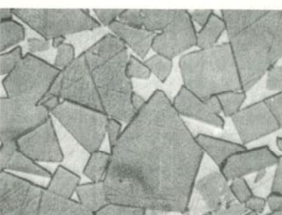
FIG.10 Comparison of microstructures at constant energy (12% cobalt; 1600X; Murakami's Etch)
